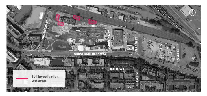
Soil investigation will include the use of a truck-mounted drill rig to collect soil and groundwater samples at various sites. All investigations will be supported by archaeology monitors from local First Nations and all soil removed will be replaced to leave the area intact.
