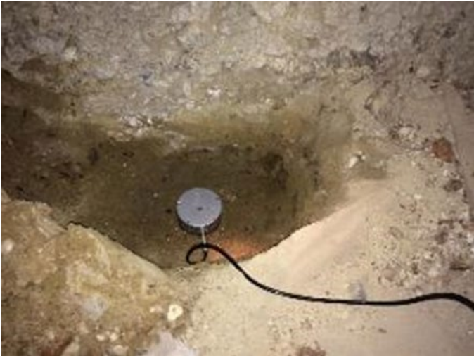
c) Transducer basement setup in soil
