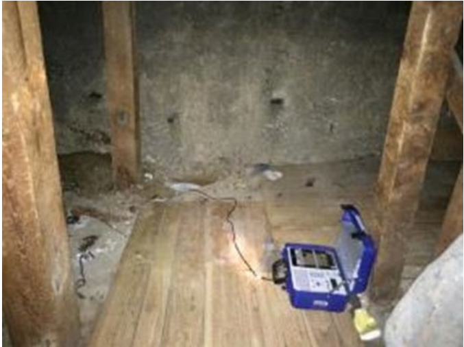
d) Blastmate III connection to transducer
