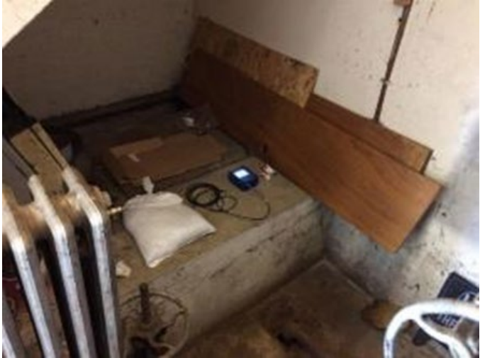
h) Micromate & Transducer sandbag setup
