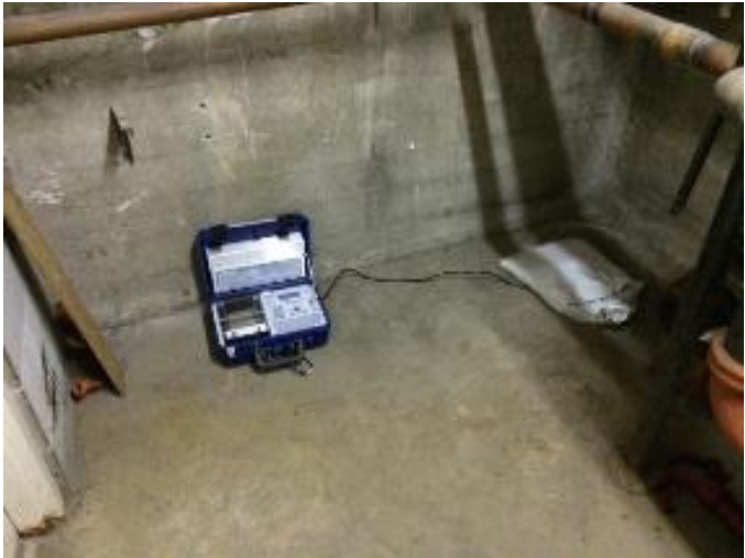
b) Blastmate III connection to transducer
