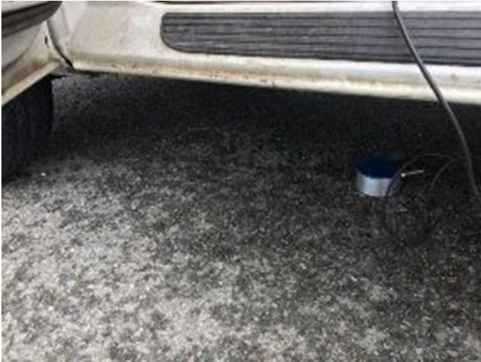
e) Transducer vehicle setup on asphalt surface
