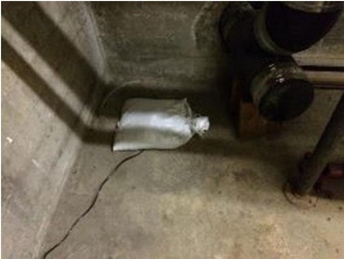
a) Transducer sandbagged on basement slab
